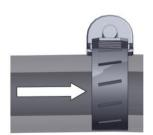
3. Slide tubing clamp over tubing and barbed portion of the fitting. Tighten clamp using a socket/nut driver or flathead screwdriver.
