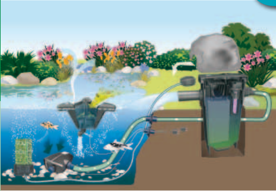
Schematic diagram: Interaction of the functions in the Clear Water System
