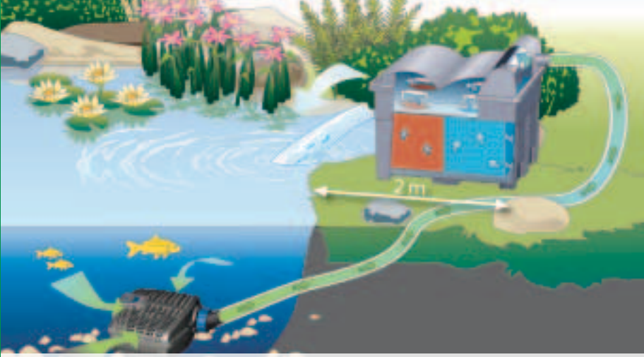
Schematic diagram: BioSmart UVC 16000 in combination with filter and watercourse pump AquaMax Eco Classic
