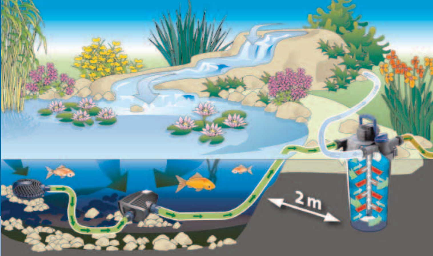
Schematic diagram: Filter and watercourse pump AquaMax Eco Premium (PRO) in combination with an OASE pressure filter FiltoClear (PRO)
