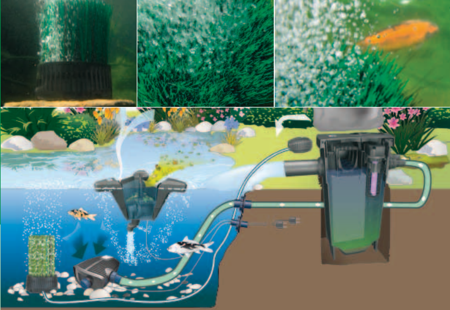
Schematic diagram: Interplay of the different components of the Clear Water System
