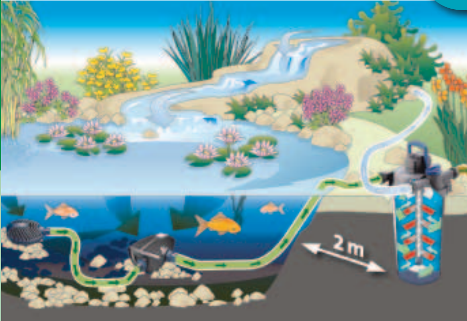
Schematic diagram: Pressure filter FiltroClear in combination with filter and watercourse pump
