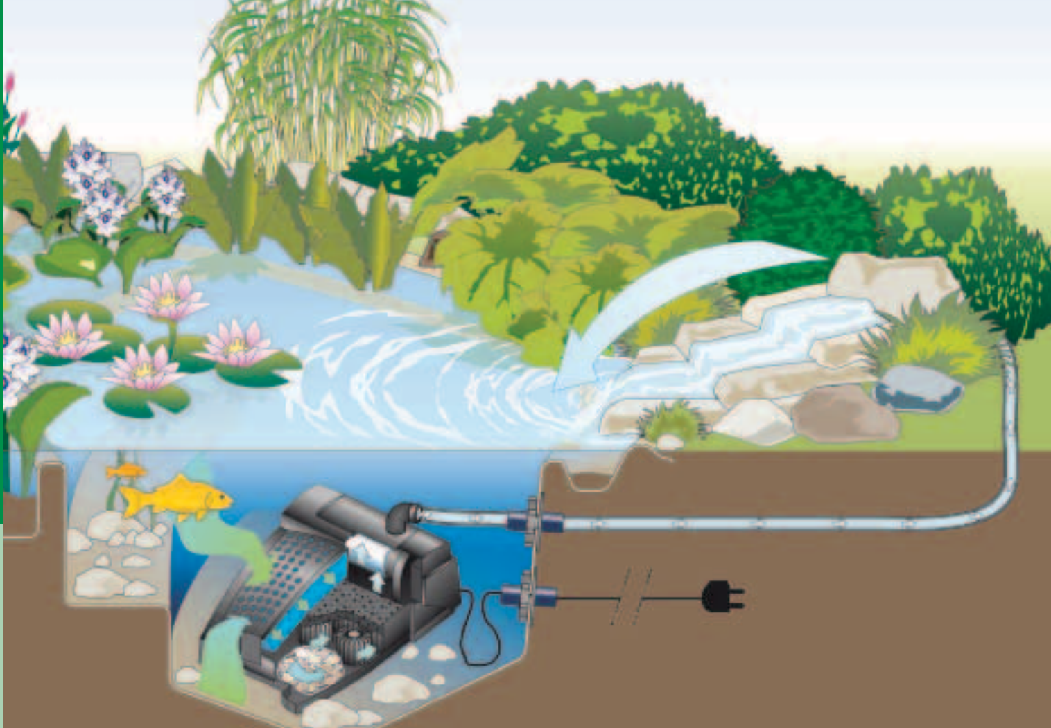
Schematic diagram: Underwater filter Filtral UVC (GB-Version) inserted in a pond
