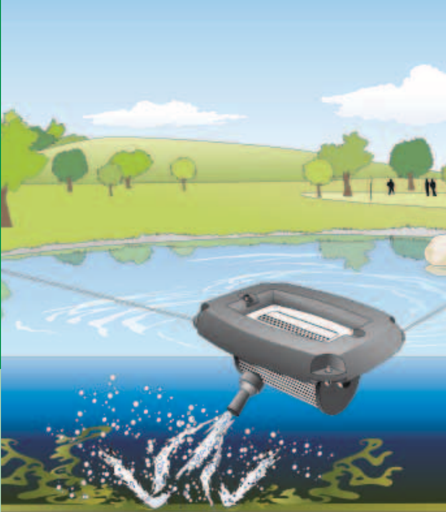
Schematic diagram: Pond aerator AquaAir 250 in use – distributes oxygen in the pond
