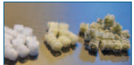
Biological surface for settlement of the microorganisms (left – biomedias that has not yet been used, right – with settled microorganisms).
