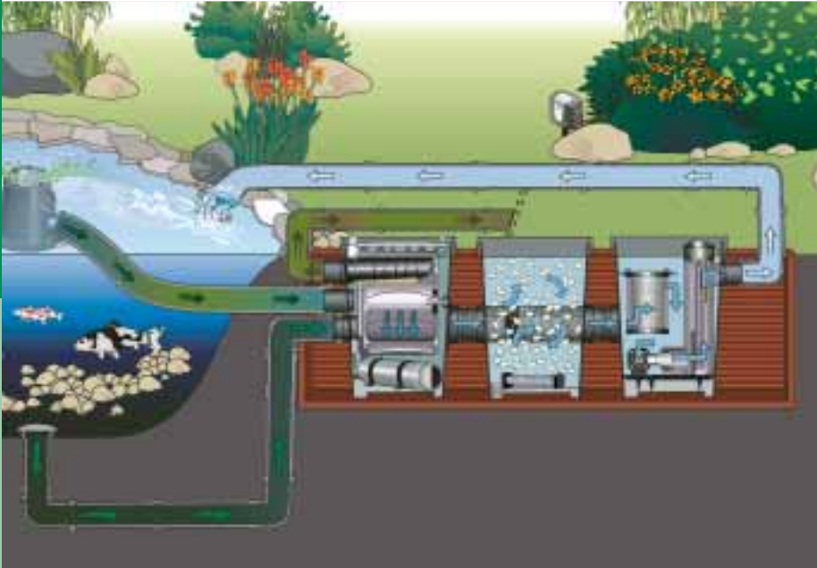
Schematic diagram: ProfiClear module filters are outstandingly suited for use on koi ponds
