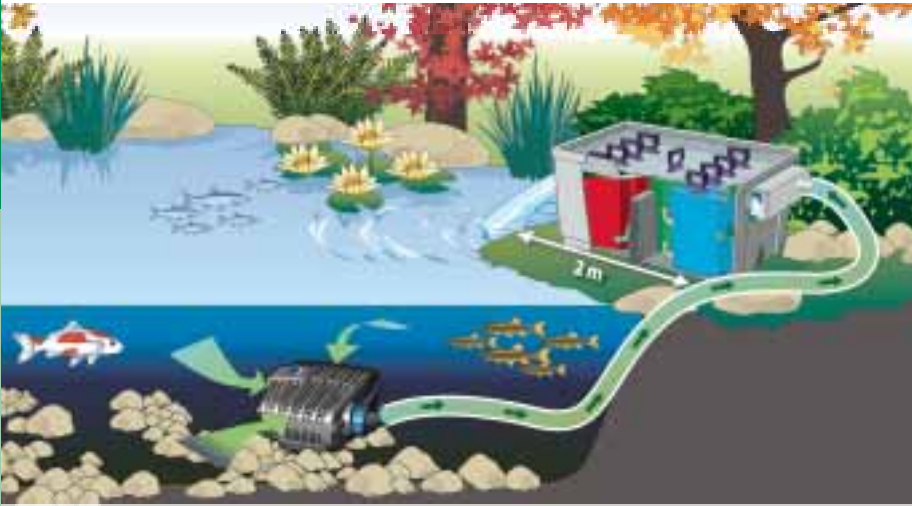
Schematic diagram: BioSmart 36000 in combination with filter and watercourse pump AquaMax Eco Classic
