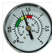
1,3 \text{ kg/cm}^2 : The pressure is 0.5 \text{ kg/cm}^2 more than the initial pressure, indicating that WASHING is required.
