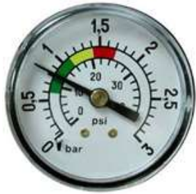
0,8 kg/cm 2 : Initial pressure of the filter at the start of a filtering cycle.
