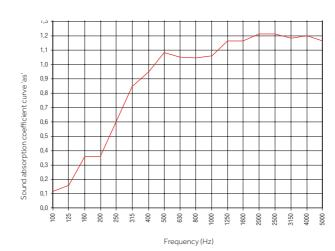
UNI EN ISO 354 measures sound-absorbing anels installed side by side and with a 200mm rear air space)
