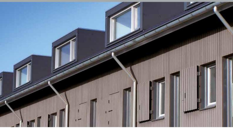
The Twinson open wall cladding system works according to the open joint principle, and combines aesthetics with functionality. The underlying structure is made of high-quality anodised aluminium, ensuring very high durability. Not only can the cladding profiles be part of a total insulation concept, they can also be used individually as finishing. Like the Twinson flat 167 wall cladding system, the elements are not only suitable for cladding walls, but also for bay windows, dormers and eaves.
