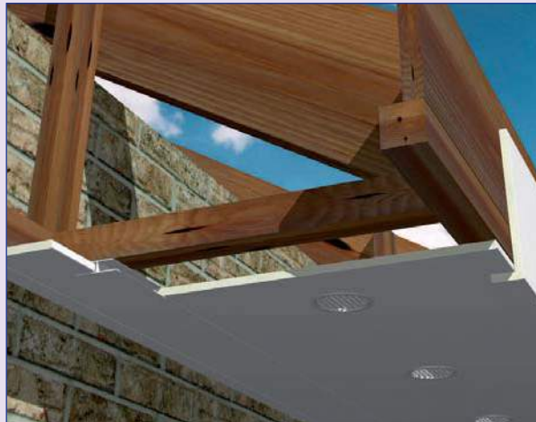
9mm Square Edge Fascia – Multi-purpose board as a Soffit vented with disc vents
