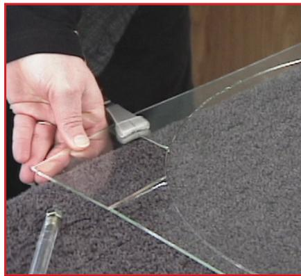
**11.** Then, run each relief score using a method or tool with which you are comfortable. Sometimes two relief scores in each corner help release the tension better.
