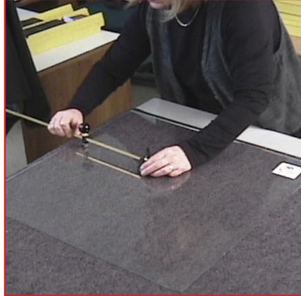
**2.** You'll score the inside of the rim first, so position your circle-cutter center, taking care to ensure that there is space enough to accommodate both the width of your border and  $1/2"$  (12mm) clearance from the edges of the sheet. Example: if you are cutting a border  $1\frac{1}{2}$ -inches (4 cm) wide, you'll need at least 2-inches (5 cm) of clearance to the sheet edge, on all sides, for the first score.
