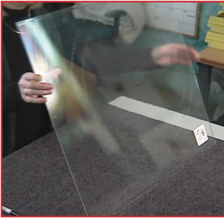
**7.** Carefully turn the sheet over so that the scored surface is down.
