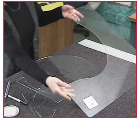
**12.** As the relief scores are run, the sheet edges should fall easily away from the circle.
