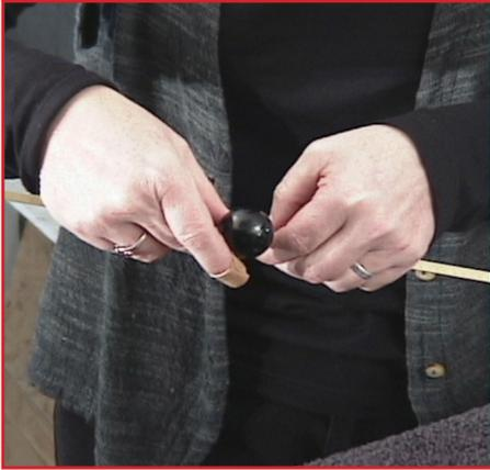
**1.** First, set your circle-cutter to  $1/32"$  (1mm) larger than the size of the center that the rim must fit around. Example: if the interior of your platter has a diameter of 17-inches, set your cutter diameter to  $17 \frac{1}{32}"$ . This tad extra allows the border to fit comfortably around your center circle.
