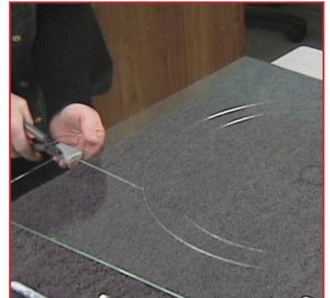
**12.** Run the relief scores one at a time, again, rotating the sheet flat on the table. Do not lift the sheet.
