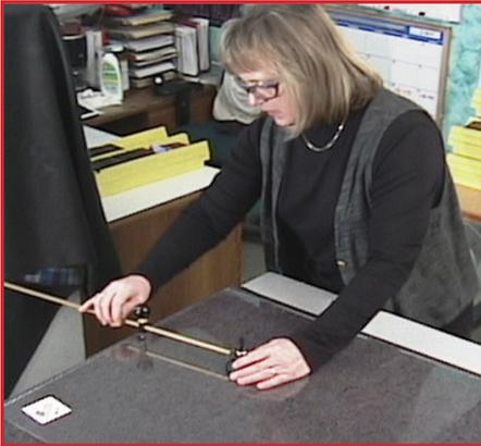
**1.** Patty locates the circle-cutter at the center of the sheet and makes sure she has at least 1/2-inch (1.25cm) clearance on all sides of the diameter of the circle.
