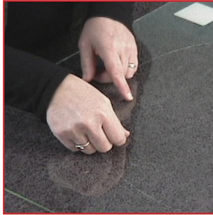
**8.** Begin running the scores by applying gentle pressure to the back side of glass, as explained in the circle-cutting demonstration. It doesn't matter which score is run first.
