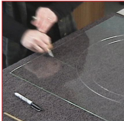
**11.** Make relief scores, drawing your glass cutter outward from the outermost circle score to the edge of the sheet. After making one, rotate the sheet without lifting it, to prevent it from collapsing under its own weight.
