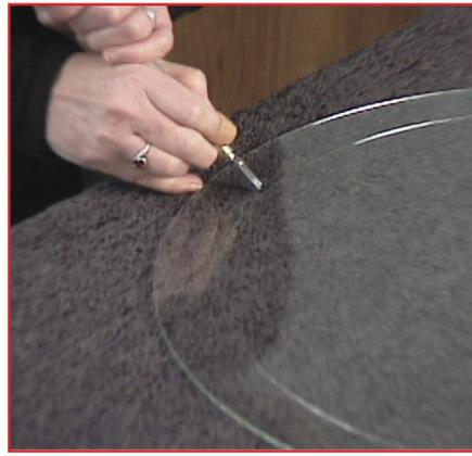
**14.** Now make a single, straight relief score outward from the interior border score to the edge of the circle, through the border. This relief score releases tension in the border "donut" and allows it to be separated cleanly from the inside.
