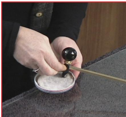
**4.** Patty oils the cutter-head before scoring. She uses a cutter oil-soaked cloth placed in a jar lid.
