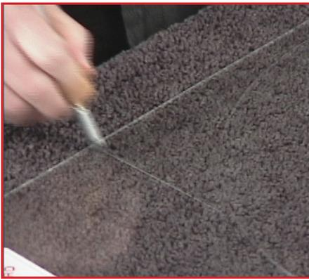
**10.** Next, make “relief” scores in the four corners of your square sheet. Each score is made away from the circle toward the edge of the sheet. Rotate the sheet flat on the table, without lifting it, to position it for making the relief scores. The sheet weakens with each score, and could break apart at any time.
