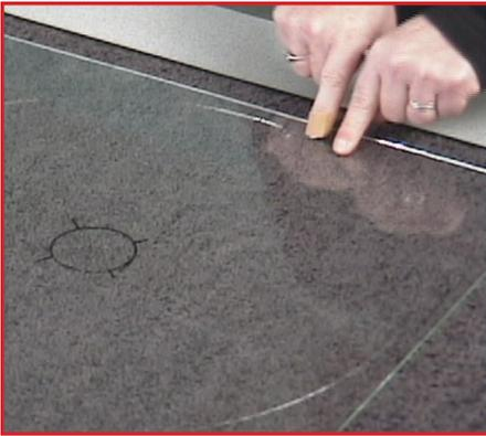
**7.** Then Patty applies pressure directly to the back side of the score. In transparent glasses, you can see the score propagate, or “run” along its path. In opal, or denser glasses, you can see a “dimpling” occur as the score runs its course.
