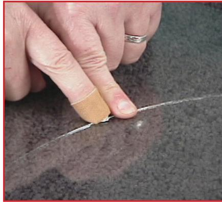
**8.** Remember to press gently. Smaller circles require more pressure, because the glass doesn't flex as easily. Seek to “run” the score completely around your circle or oval. Press over the score line a few times, all the way around, until you are satisfied the “run” is complete.
