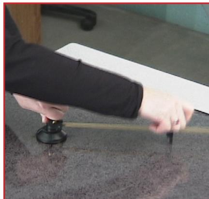
**5.** She rotates the cutter-arm, scoring the glass 360° in a smooth motion with even pressure. Then, she removes the circle-cutter.
