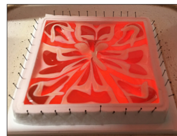
The same piece as above shown red-hot in the kiln immediately after combing. Note that you can see Patty's ceramic fiber damming technique in both these photos.
