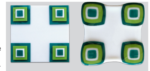
Left: Strictly for the sake of demonstration, we created a single-thick square of glass with smaller square stacks in each corner. Right: After Full Fusing, the thin areas draw in; the thicker areas push out as the uneven layers seek equilibrium.
