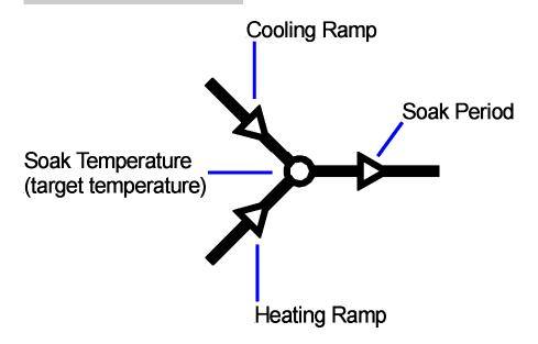
A KCR32C firing segment comprises a ramp followed by a soak period. Two segments can be used for simple firing (biscuit firing for example) or several segments can be used per program for complex firing (crystal glazing or glass-making for example).
