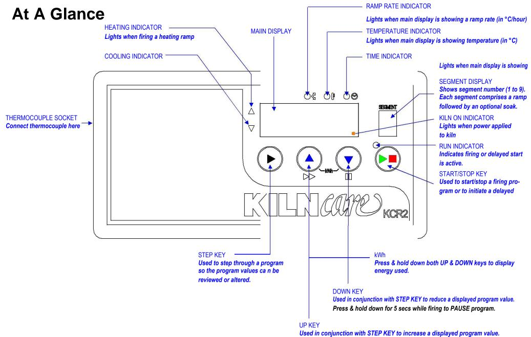
Press & hold down for 5 secs while firing to ADVANCE program.
