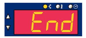
Explanation: the full range of displayed values for ramp rate are: End, 1...999°/hr, FULL. To mark the end of a program select a ramp rate of "End" by holding down the ▼ key until End is displayed. To add an extra segment press the ▲ key until your de-sired ramp rate is shown. If you want to heat at full power hold down the ▲ key until FULL is displayed.
