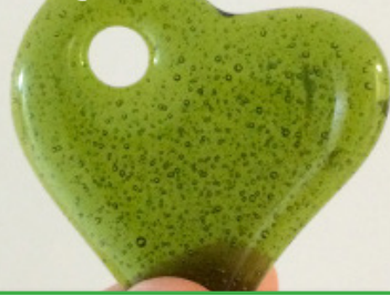
Image 3: Filled using only medium grain frit. Still bubbles, but much clearer overall.
